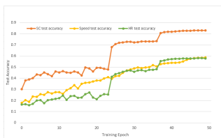
Figure 4: An Overview of Test Accuracy between skin conductance (Orange), heart rates (Green) and Vehicle Speed (Yellow).
